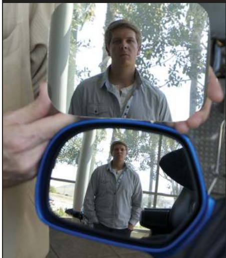
REGULAR MIRROR (ABOVE) AND CONVEX MIRROR (BELOW)
