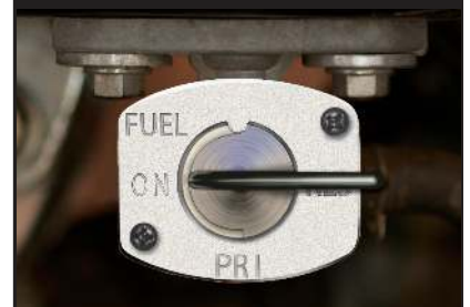
FUEL SUPPLY VALVE WITH PRIME
